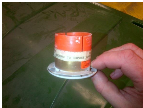
Concealed sprinkler extended due first fix fitout height error
