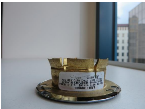
Concealed Sprinkler Butchered to fit a standard spray sprinkler.
