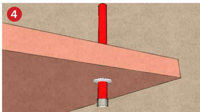
Cable through a Plasterboard ceiling with Fire rated Mastic applied
