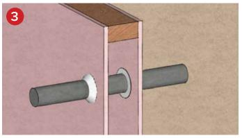
Metal pipe with Fire rated Mastic applied
