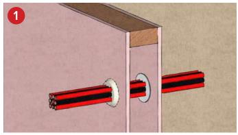
Cables with Fire rated Mastic applied
