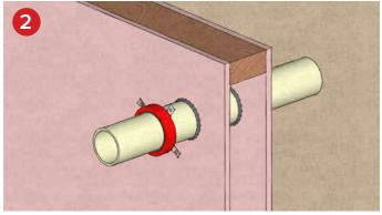
Fire collar with Mastic applied at wall prior to install of collar
