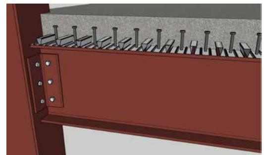
**Figure 4: Re-entrant or ‘dovetail’ profiled decking**
