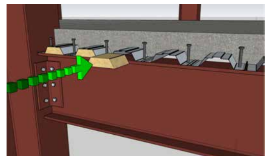
Figure 3: Filling voids in trapezoidal profiled decking
