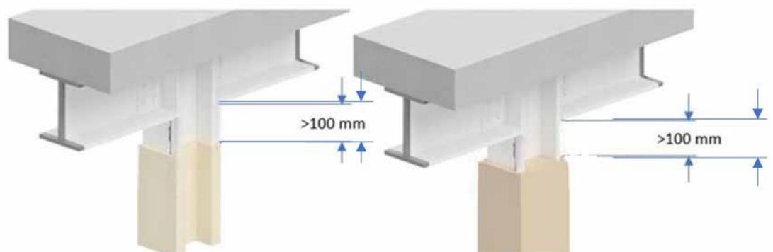
**Figure 1: Left - Junction between cementitious (column) and intumescent coating (beam).
