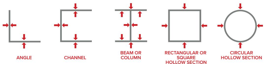
**Figure 6: Pictorial guide for locations of DFT readings**
