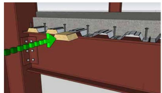
**Figure 3: Filling voids in trapezoidal profiled decking**
