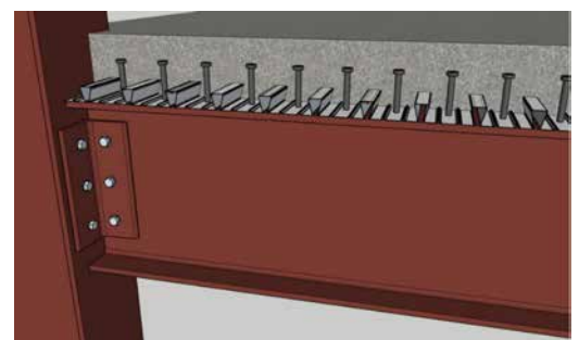
Figure 4: Re-entrant or ‘dovetail’ profiled decking
