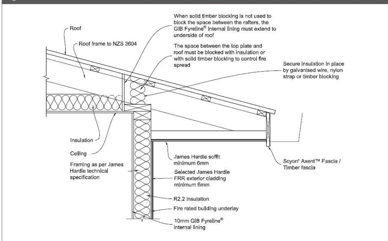
A manufacturer's specification showing soffit installation which maintains fire separation.
