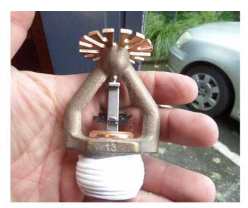
All sprinkler manufacturers recommend a maximum torque that sprinklers can be tightened too. Overtightening a sprinkler can lead to leakage, or even catastrophic failure.
