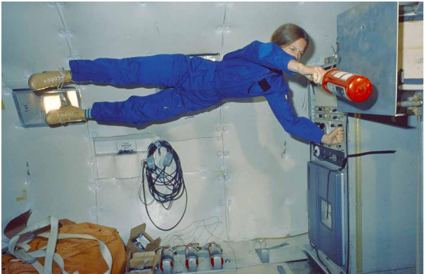
*Astronaut Marsha Ivins on the KC-135 performing a Zero G evaluation of orbiter fire extinguishers.*
