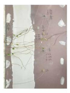
LEFT: Steel studs glow red-hot immediately following a pilot-scale furnace test. MIDDLE: A timber framed specimen at the end of a full-scale furnace test. RIGHT: Thermocouples collect important temperature data.
