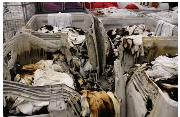
Bins of towels where the fire occurred, and was contained by the sprinklers.
