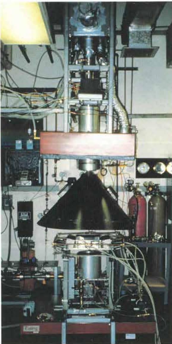
The Small-Scale Flammability Apparatus will be used to examine the nonthermal fire damage potential of materials found in electronics and textiles. (See Figure 1 on page 2 for a diagram of the apparatus.)
