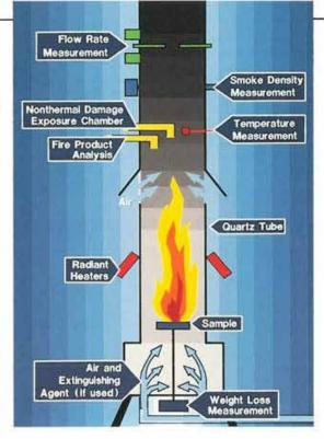
Figure 1. An exposure chamber attached to the sampling duct at the area marked "Nonthermal Damage Exposure Chamber" will contain the sample items to be tested.
