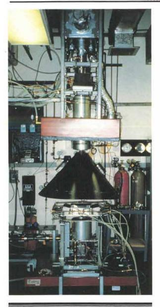
The Small-Scale Flammability Apparatus will be used to examine the nonthermal fire damage potential of materials found in electronics and textiles. (See Figure 1 on page 2 for a diagram of the apparatus.)
