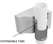
On the underside of the substrate, the TD Collar may be exposed no more than 80mm, or be recessed no more than 10mm.
