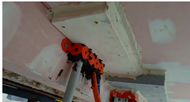
Above: FyreSTRAP installed in a full scale wall fire test Below: FyreSTRAP installed in a ceiling fire test with an adjacent wall
