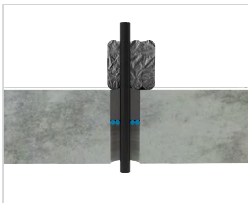
FyrePEX TM HP Sealant applied to the correct fill depth.
