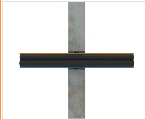
FyrePEX TM HP Sealant to be filled to depth specified. Refer to service specific requirements on page 6 .
