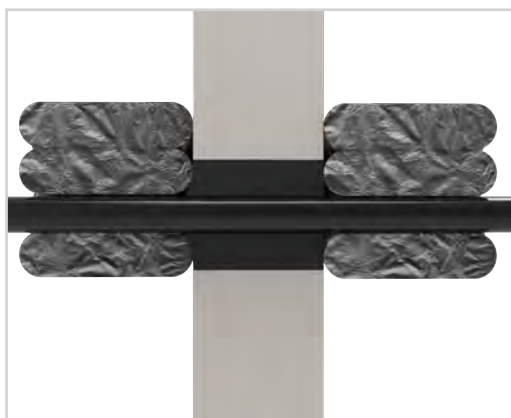
FyrePEX TM HP Sealant applied to the correct depth of the wall.
