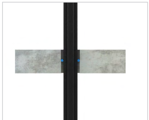
FyrePEX TM HP Sealant installed into Slab opening to a depth of at least 60mm from one side only. Refer to service specific requirements on page 9 .
