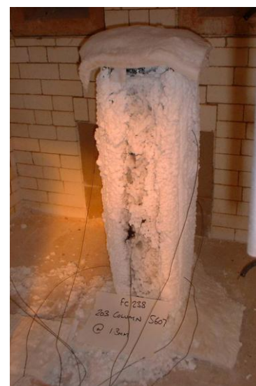
Figure 13 Example of intumescent column (short section) test
