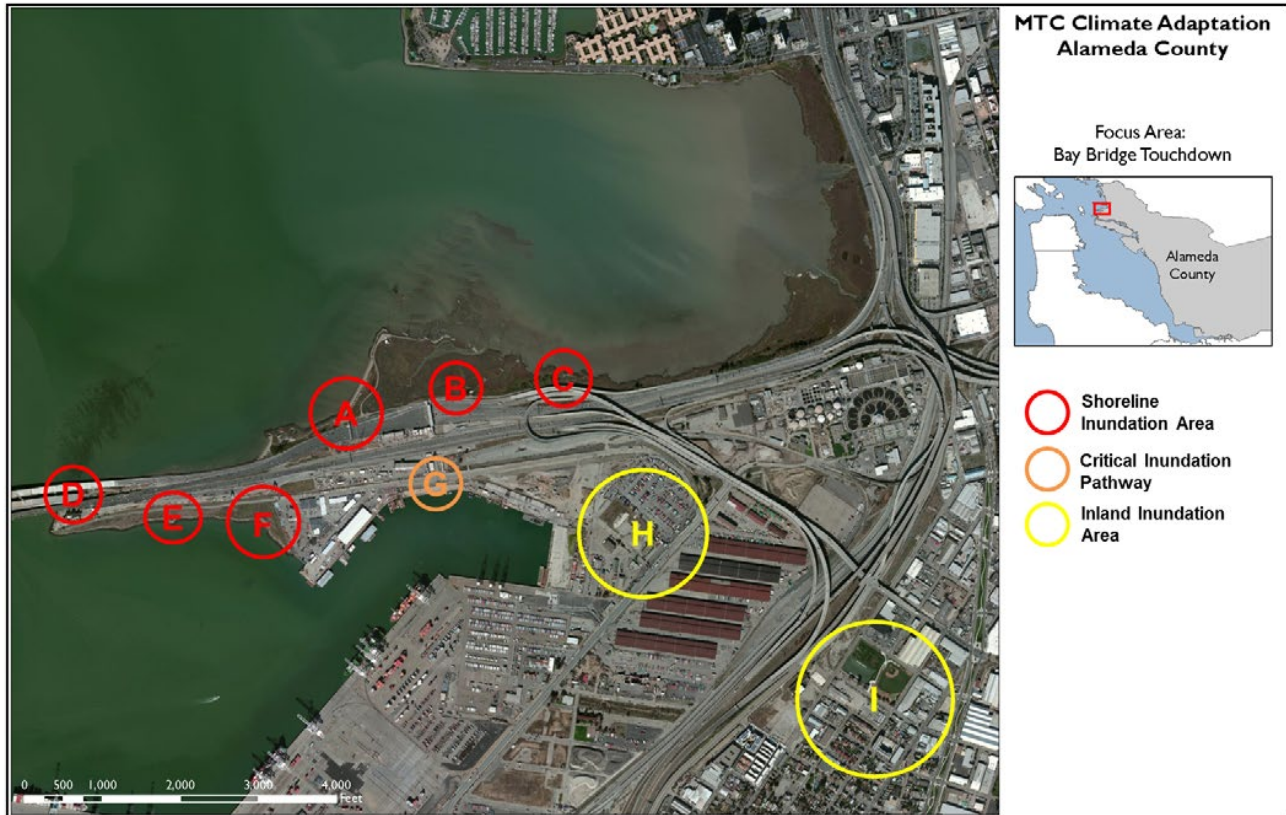
Figure 7: Example of Failure Point: Critical Inundation Pathway Connecting Shoreline Inundation Areas to Inland Inundation Areas
